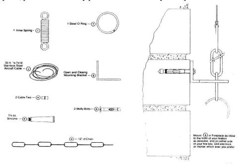
on the edge of tile. CAUTION: Pay special attention to not over-tighten the three set screws on the mounting bracket. Over-tightening will crack the ceramic flue tile. Also, the set screws should be loose enough to allow the bracket to tilt slightly inward so that there will be little or no gap where the ASCC meets the flue tile on the side opposite the mounting bracket.
